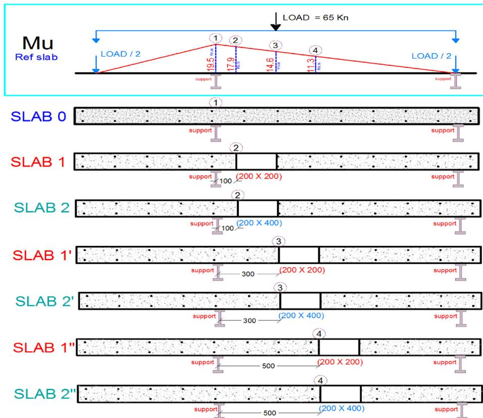
Fig. 20 Position of cutouts in hogging region, quarter and mid span.
