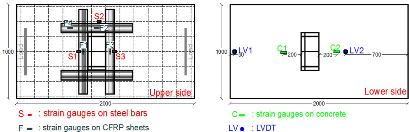
**Fig. 3** Measuring instruments (strain gages and LVDTs) on the sides of the tested slabs.
