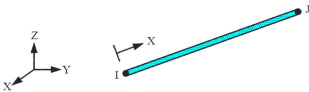
**Fig. 13** LINK180 element geometry, ANSYS (2011).
