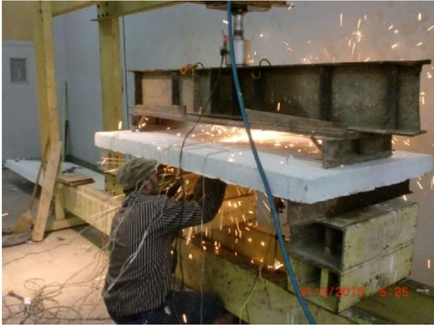
Fig. 5 Cutting concrete and steel bars.
