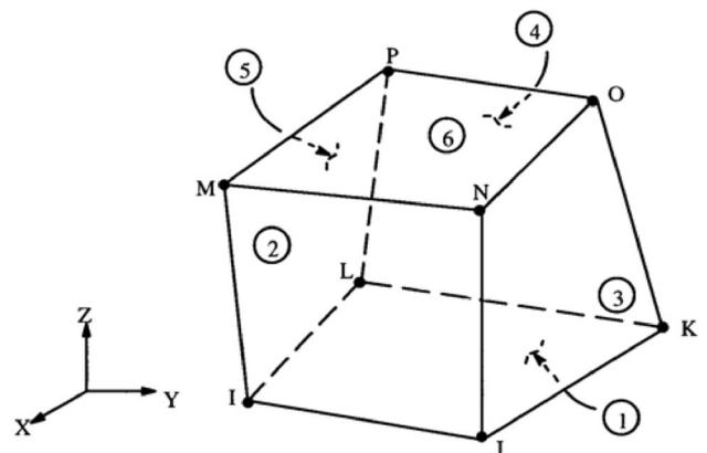
Fig. 11 SOLID 65 3D-reinforced concrete solid element, ANSYS (2011).
