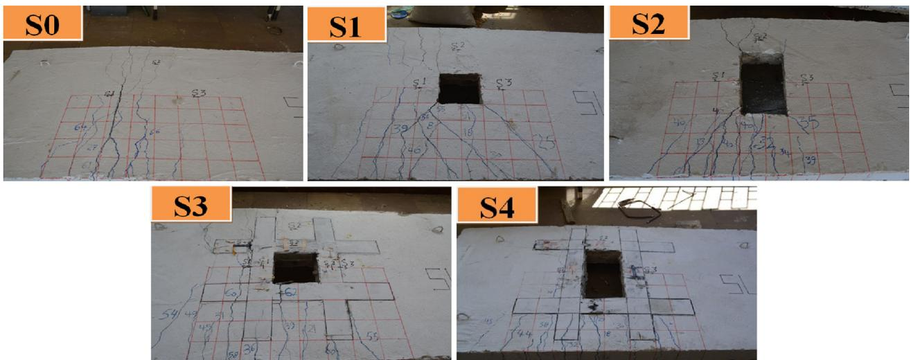
Fig. 6 Crack patterns of tested slabs.
