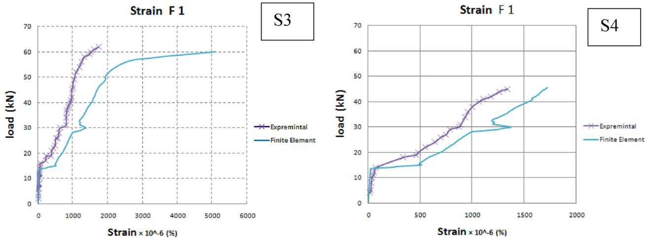
Fig. 18 Load-strain history in the longitudinal direction (F1) of slabs S3 and S4.
