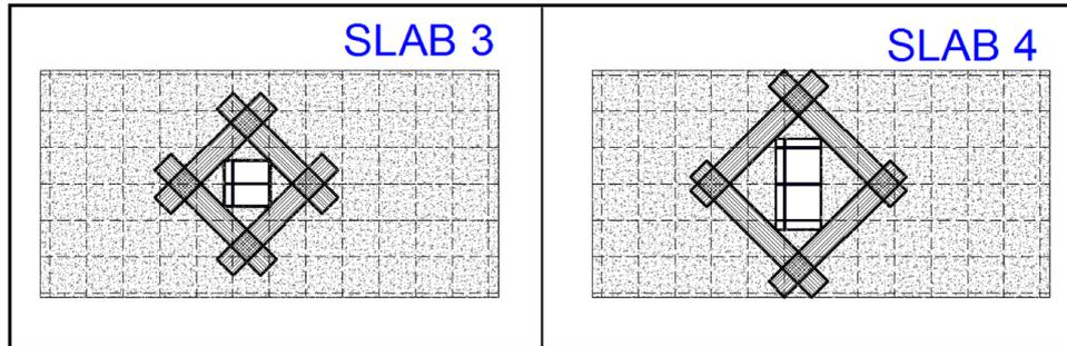
**Fig. 21** Strengthened slabs with CFRP sheets with 45°.
