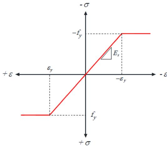
Fig. 15 Stress-strain curve for steel reinforcement.
