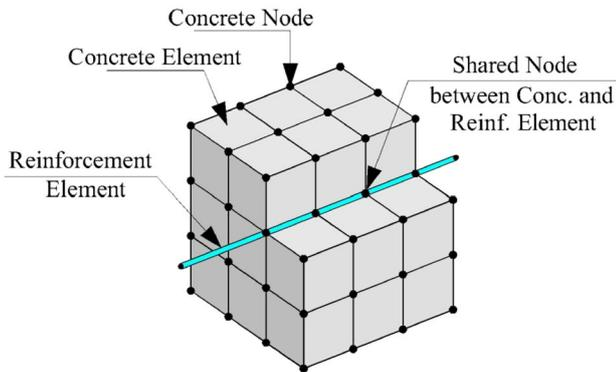
Fig. 10 Discrete model for reinforced concrete (ANSYS).
