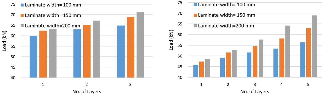
Fig. 19 Effect of CFRP layers for slab groups 1 (left) and 2 (right).
