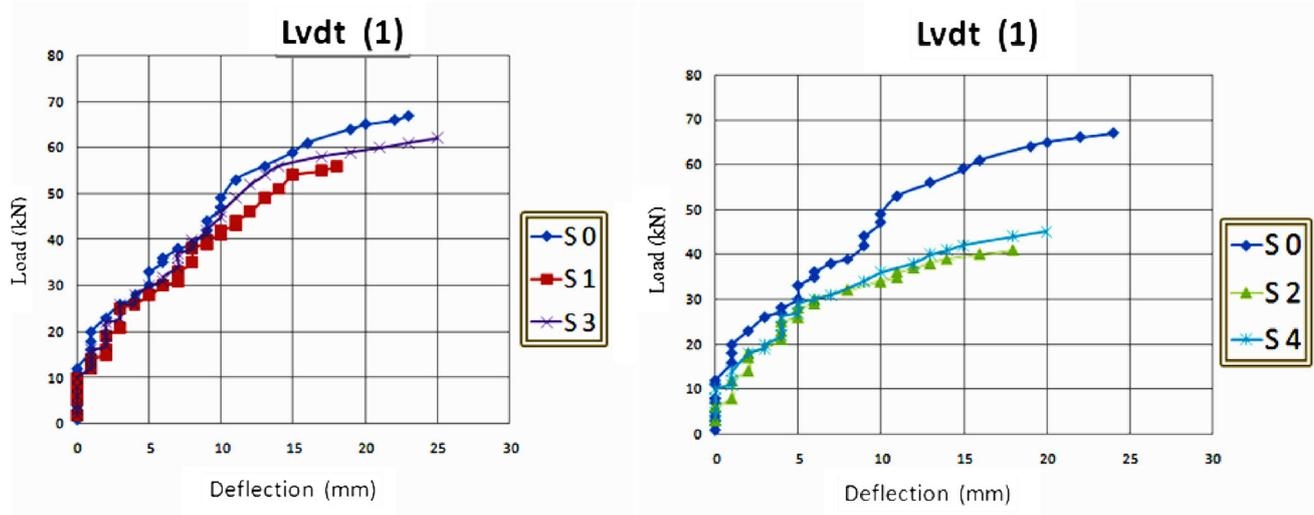
Fig. 7 Load-deflection curves for tested slabs.
