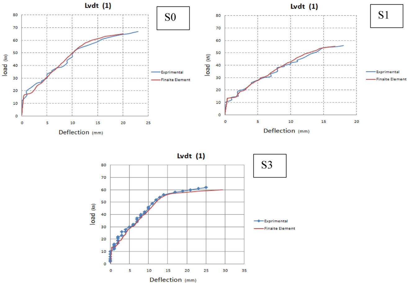
**Fig. 17** Load-displacement history of slabs S0, S1, and S3.
