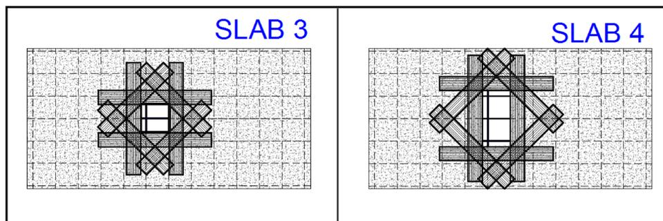
**Fig. 22** Strengthened Slabs with CFRP sheets with 90° and 45°.
