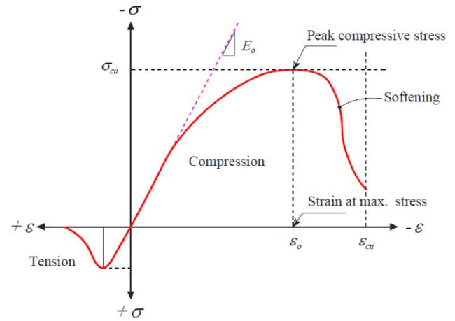
**Fig. 14** Typical Uniaxial Compressive and Tensile Stress-Strain Curve for Concrete, Bangash, (Mota and Kamara 2006).
