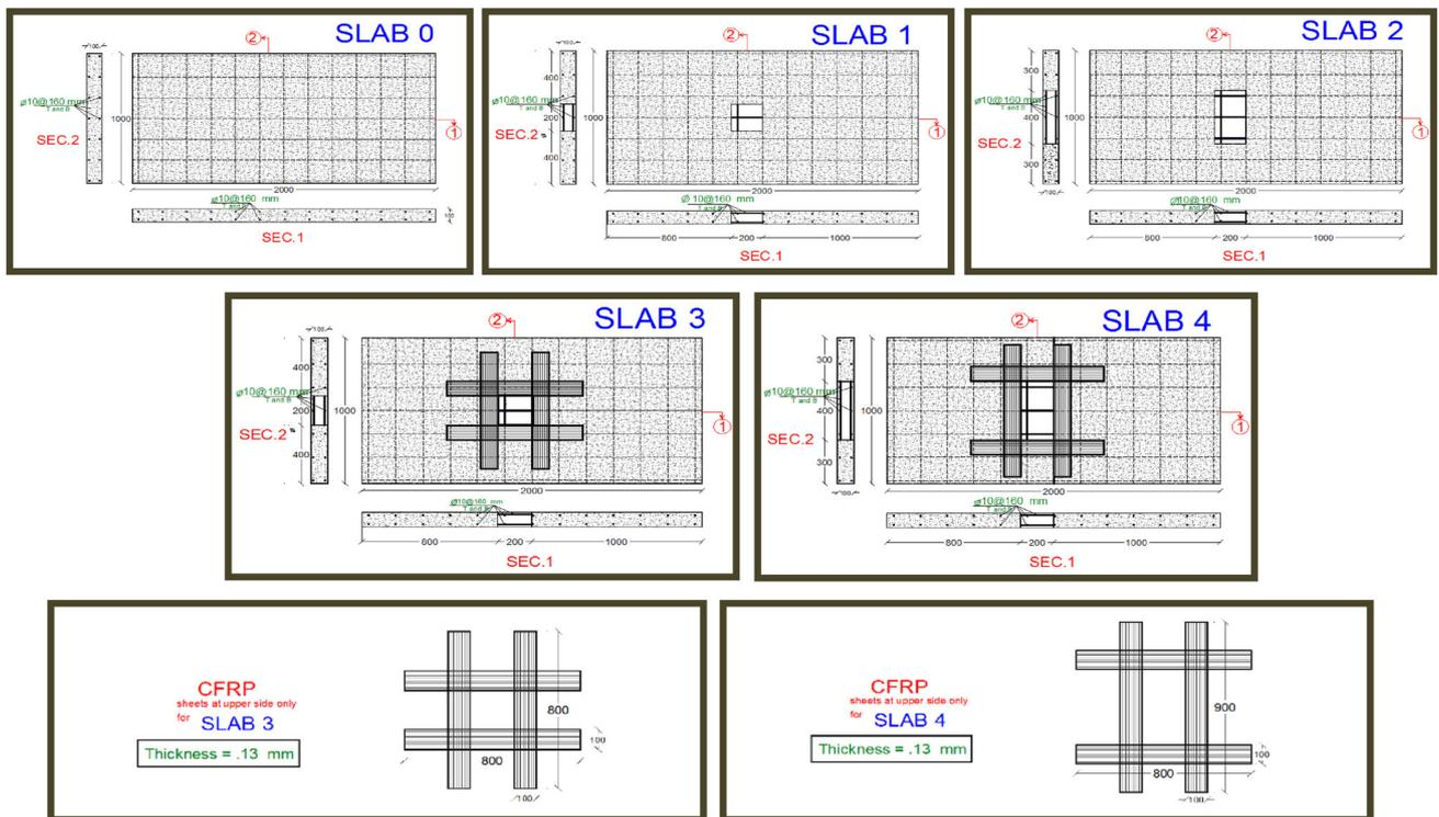
**Fig. 2** Details of tested specimens.
