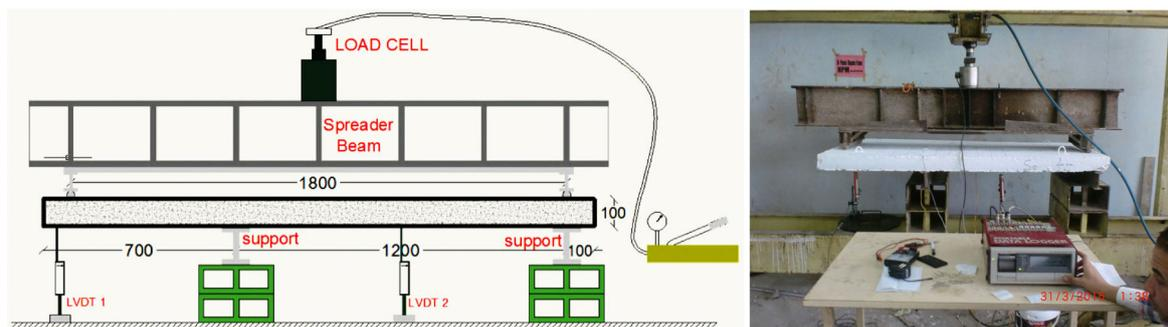
**Fig. 4** Loading arrangement and test setup.
