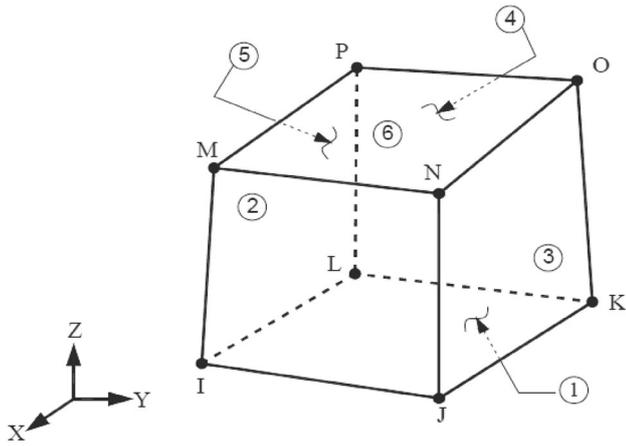
**Fig. 12** SOLID185 3D- Homogeneous Structural solid element, ANSYS (2011).
