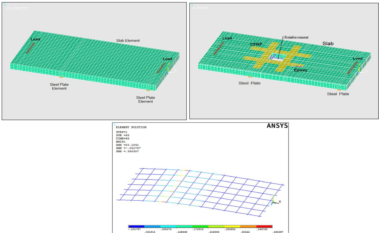
Fig. 16 FE model of the control slab, slab (1), and reinforcement mesh.
