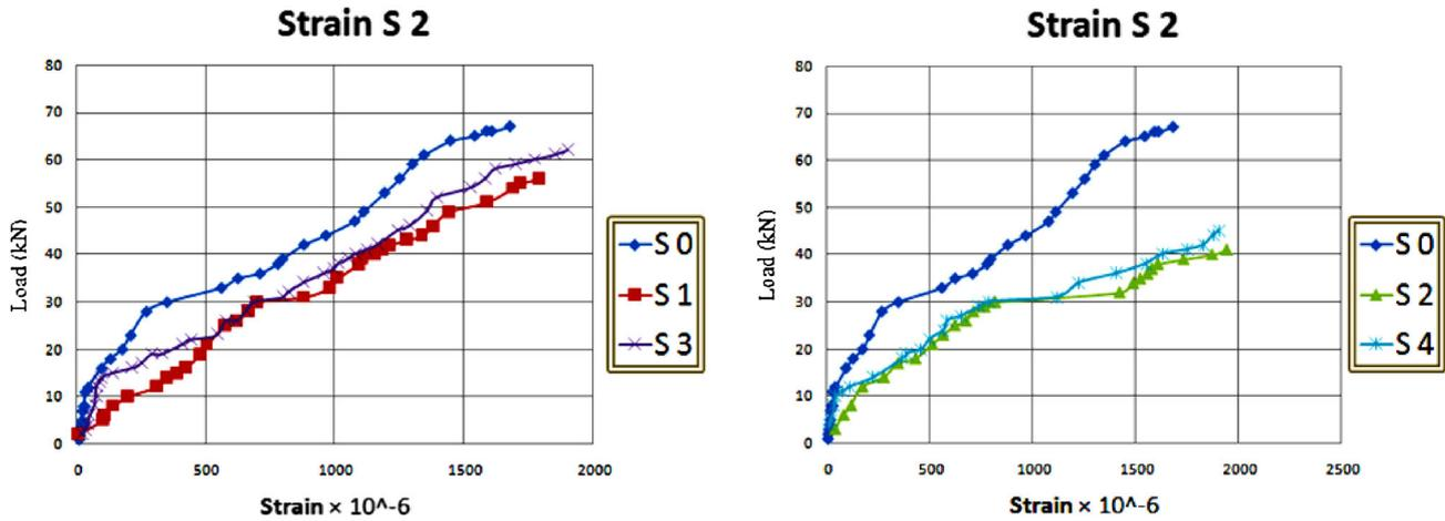
Fig. 8 Load-strain curves for steel bars of tested slabs.
