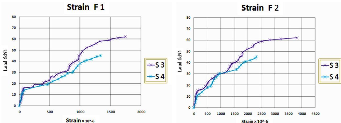
Fig. 9 Load-strain curves for CFRP sheets of strengthened slabs.
