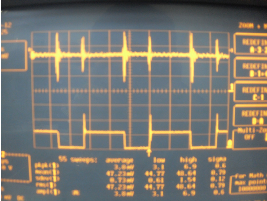
Fig. 6. Converter switching waveform of fuel cell simulator (upper trace : output current : 1 A/div, lower trace : switching voltage 20 V/div)
