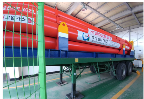
Fig. 4. Tube trailer in Naepo HRS in chungnam province
