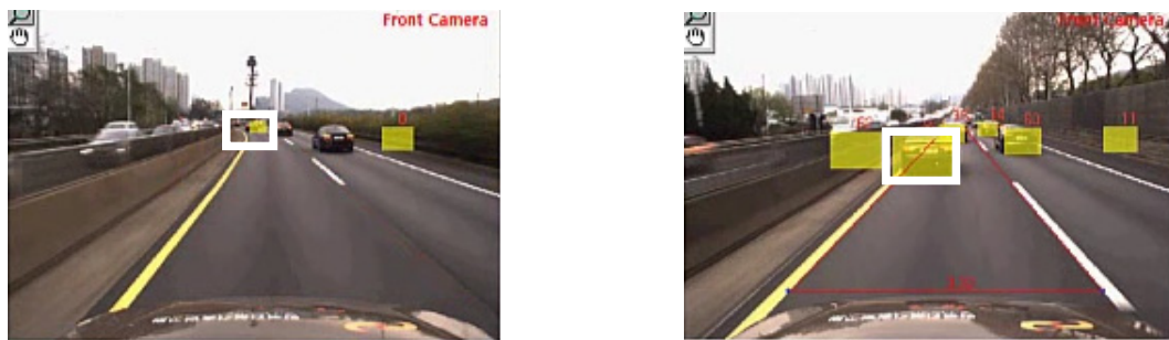
Figure 2. Data acquisition from survey vehicle(L: Circular, R: Tangent)
