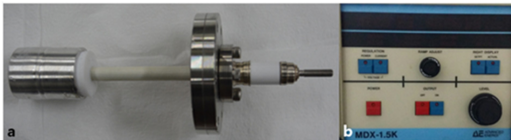
Fig. 4. Photograph of composed feed-through and DC power supply.
