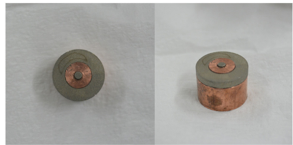
Fig. 1. Magnet array cathode (Sm-Co side magnet : D20×d13×3T, center magnet : D5×5T mm).
