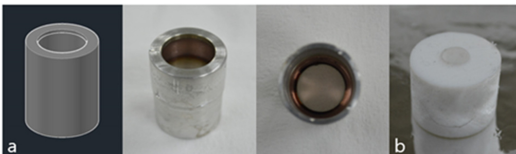
Fig. 3. Photograph of anode cover and teflon joint (a : Anode cover, b : Teflon joint).
