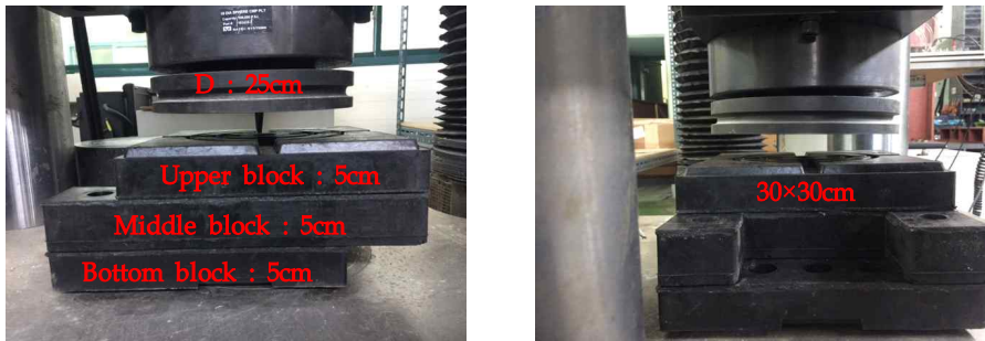
Fig. 4. Compression test of lego block system
