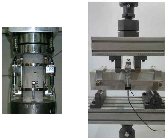
(a) Compressive test (b) Flexural test Fig 2. Test set up of mechanical properties
