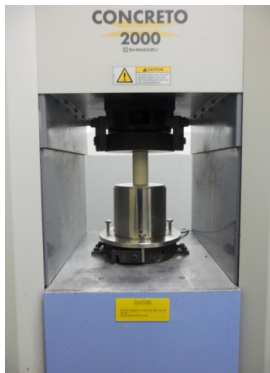
Fig. 3. Uniaxial direct compressive test of granite
