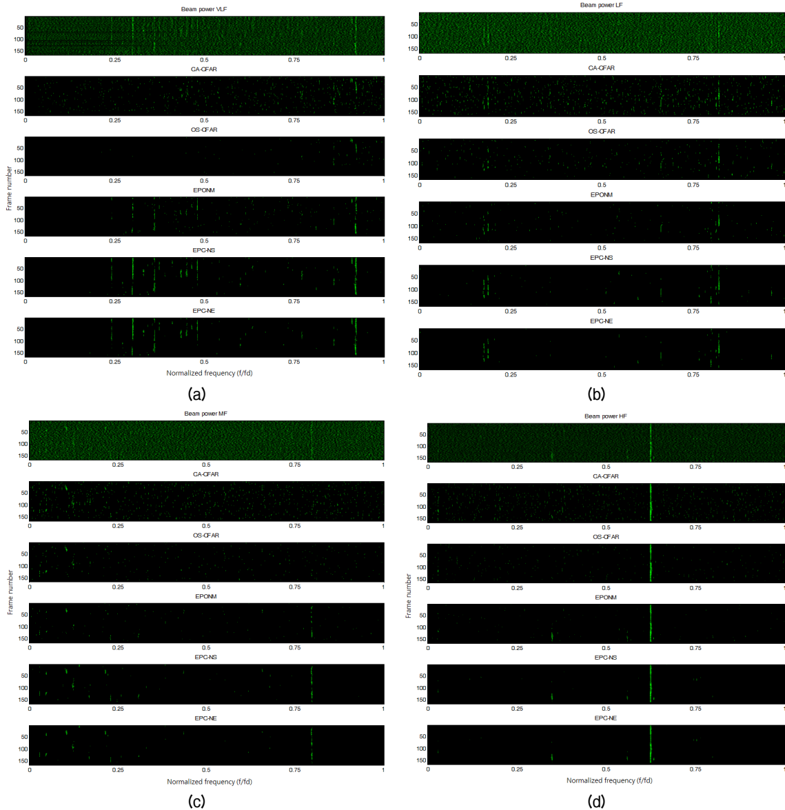
Fig. 9. Lofargrams of real ocean acoustic data for four frequency bands: (a) VLF, (b) LF, (c) MF, and (d) HF.
