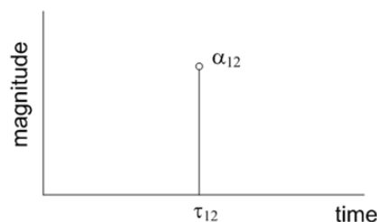
Fig. 3. Time delay channel model between two received signals.
