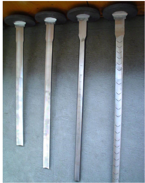
Fig. 3 Experimental chevron defects found in open-die extrusion process
