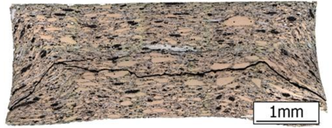
Fig. 1 Cross-section of shock compacted Ni/Al
