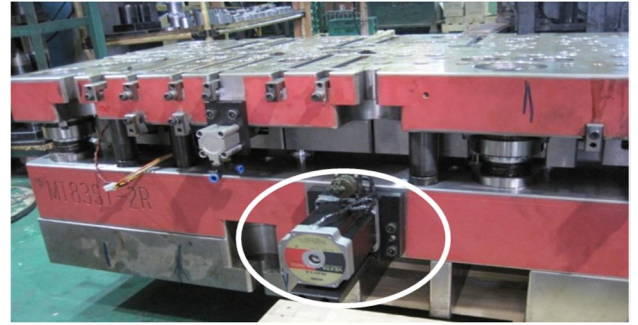
Fig. 4 Skew motor of motor core laminated stamping die
