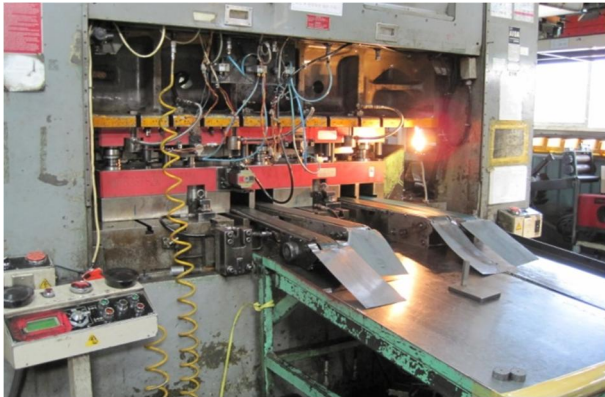
Fig. 7 Press tryout of motor core laminated stamping die
