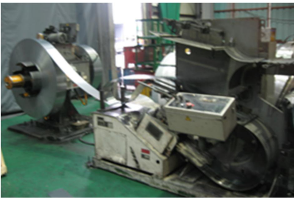
Fig. 8 Uncoiler, leveller, loop control arm for producing motor core
