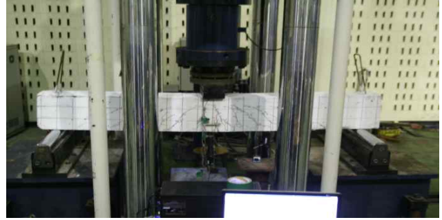
Figure 7. Flexural behavior testing of RC beam
