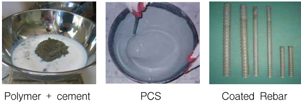
Figure 1. Making of PCS-coated rebar 11)
