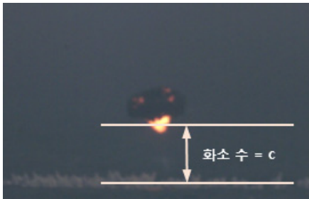
Fig. 4. HOB measurement of sea impact test
