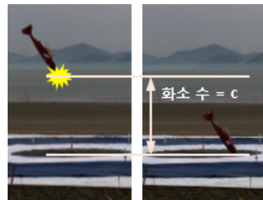
Fig. 9. HOB measurement of ground impact test
