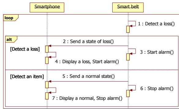
Fig. 7. Sequence Diagram of Sensing Loss of Items
