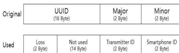
Fig. 8. Data Structure for Sensing Loss of a Smartphone
