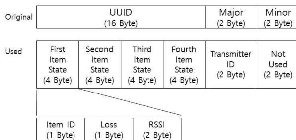
Fig. 6. Data structure for Sensing Loss of Items
