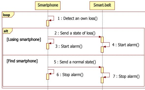
Fig. 9. Sequence Diagram of Sensing Loss of a Smartphone
