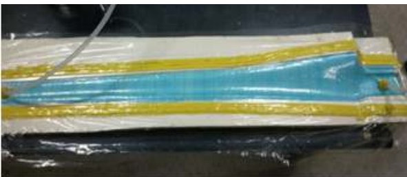
(b) Resin injection process
