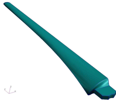
Fig. 2 Designed aerodynamic configuration of wind turbine blade
