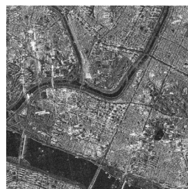
Fig. 2. COSMO-SkyMed 2 image with speckle noise removed using Gamma-MAP filter
