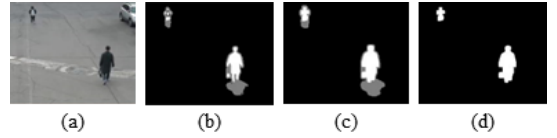
(Figure 2) This is the RGB-based segmentation result. (a) Input image (Left). (b) Mixture of Gaussians. (c) Morphology. (d) Binarization.
