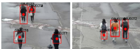
(Figure 7) The result of tracking with CAMShift using RGB-D model
