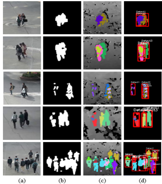
(Figure 6) This is the object detection result using RGB-D information. (a) Frame. (b) RGB-based segmentation. (c) Depth-based segmentation. (d) Object Detection.
