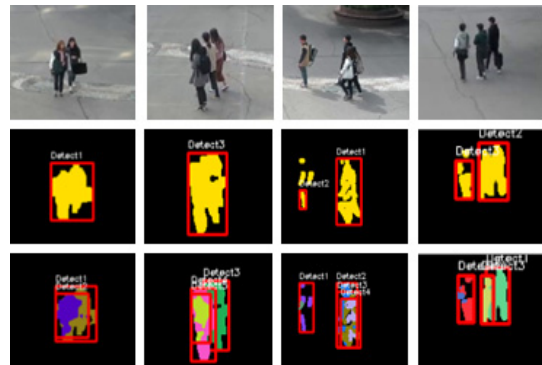
(Figure 8) This is the result of comparing object detection methods. (Top) Input image. (Middle) Object detection using only RGB information. (Bottom) Object detection using RGB-D information.
