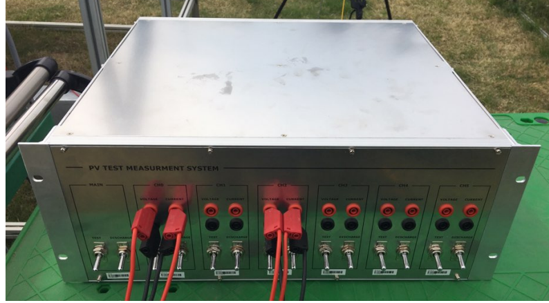
Fig. 4 Prototype of developed multi-channel array tester
