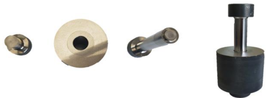
Fig. 12 Prototype net shape mold
