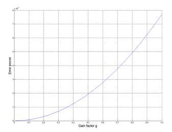
Fig. 6. Variation in the power of the error signal in terms of gain for one noncoherent interference case.
