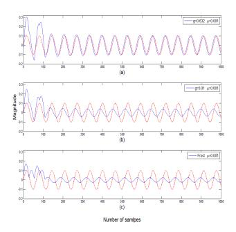
Fig. 3. Comparison of array output and desired signal for two coherent interference case for  $1 \le k \le 1000$ .
