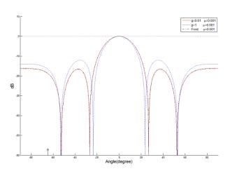
Fig. 9. Comparison of beam patterns for one noncoherent interference case.
