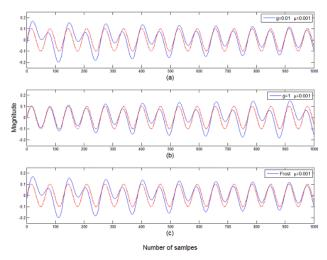
Fig. 7. Comparison of array output and desired signal for one noncoherent interference case for  $1 \le k \le 1000.$
