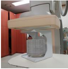
[Fig. 2] NEMA Phantom's diagonal arrangement between tube and detector
