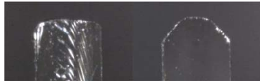
Fig. 3. Cross sections of sapphire wafer edge before and after grinding.
