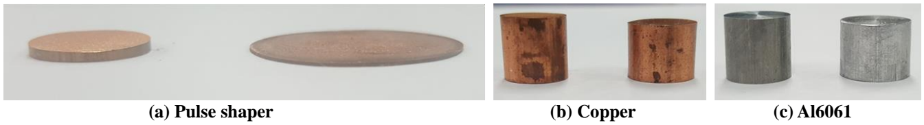
Fig. 7 Shape before and after deformation of pulse shaper and specimen
