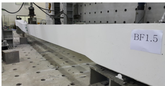
Fig. 19. Failure pattern of BF1.5-14 in central section
