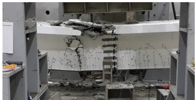
Fig. 18. Failure pattern of CFS1.0
