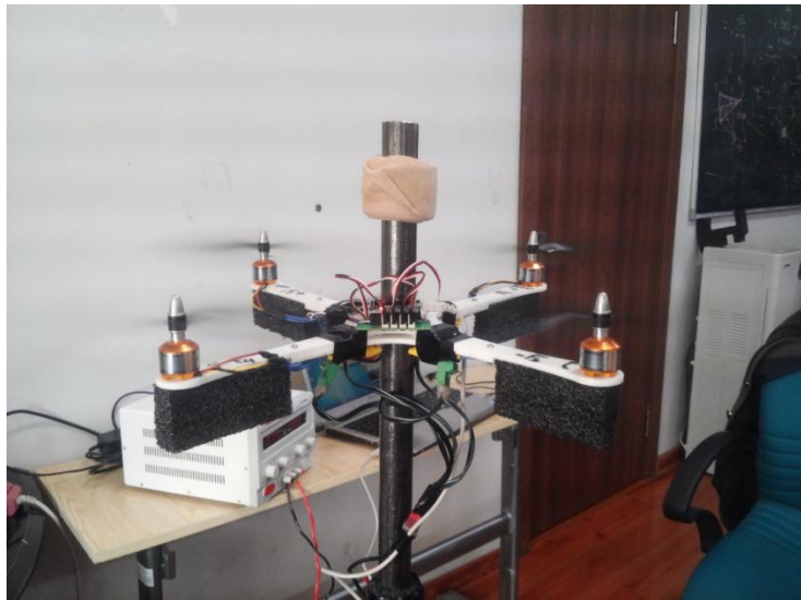
Figure 5. The experimental environment of the quadcopter system.
