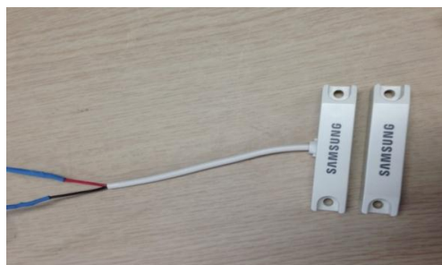
Figure 4. Door Control (SIM-0001 Sensor)
