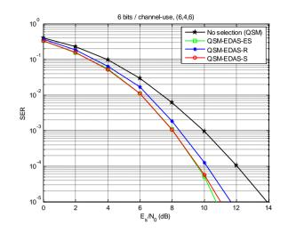
Figure 3. SER performance comparison of QSM-EDAS-ES, QSM-EDAS-R, and QSM-EDAS-S algorithms for  $N_T = 6$ ,  $N_S = 4$ , and  $N_R = 6$
