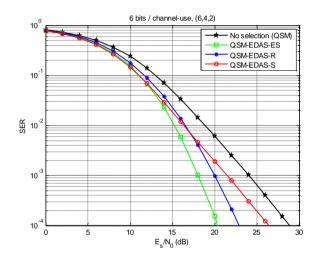
Figure 1. SER performance comparison of QSM-EDAS-ES, QSM-EDAS-R, and QSM-EDAS-S algorithms for  $N_T = 6$ ,  $N_S = 4$ , and  $N_R = 2$
