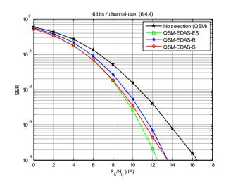
Figure 2. SER performance comparison of QSM-EDAS-ES, QSM-EDAS-R, and QSM-EDAS-S algorithms for  $N_T = 6$ ,  $N_S = 4$ , and  $N_R = 4$
