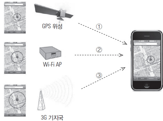
Fig. 1. Location positioning method of smartphone(4)
