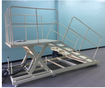
Figure 2. Variable stair walkway
