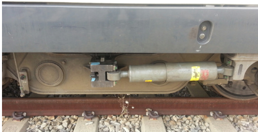
Fig. 3. Yaw damper installation change
