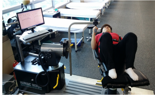
Fig. 1. Measurement of the computer assisted isokinetic muscle strength in the elbow joint
