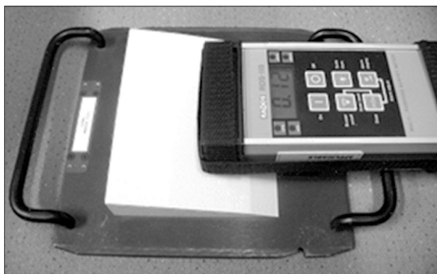
Fig. 1. Measurement of dose rate using GM detector and activated wedge filter.
