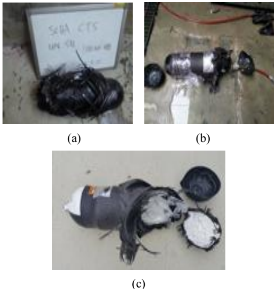
Fig. 7 Failure modes of the sample cylinders as a result of burst tests with (a) iso-dome; (b) prolate; and (c) oblate cylinders
