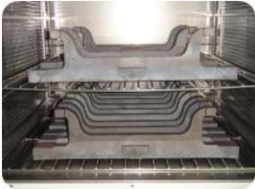
Fig. 9 Thermal shock test setup
