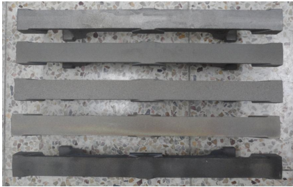
Fig. 4 Coated grate bar with four materials
