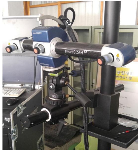
Fig. 6 3D scanner for measuring deformation
