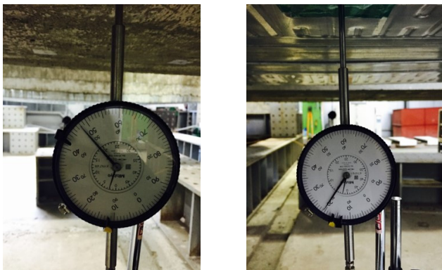
Fig. 11 Dial gauge shape for measuring deflection
