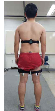
Figure 2. Location of the electrodes and myomotion sensors.
