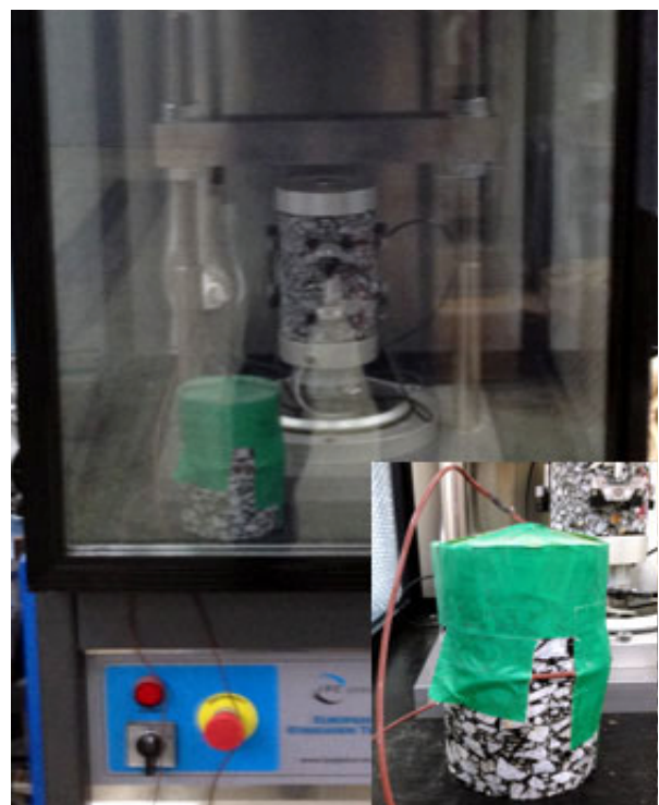
Fig. 1 Cylindrical Specimen with Thermocouple in a Temperature Conditioning Chamber
