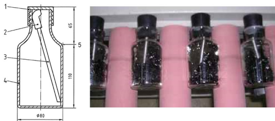
Fig. 4 Dynamic Immersion Test
