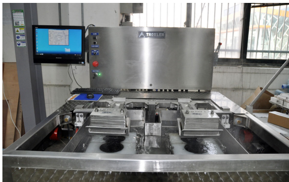
Fig. 6 Hamburg Wheel Tracking Test Machine
