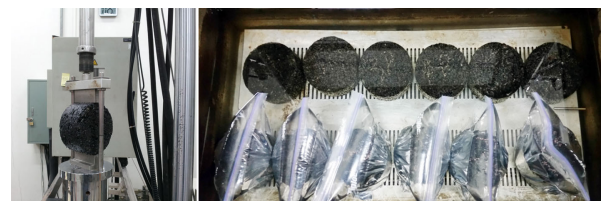
Fig. 5 Indirect Shear Strength Ratio Test
