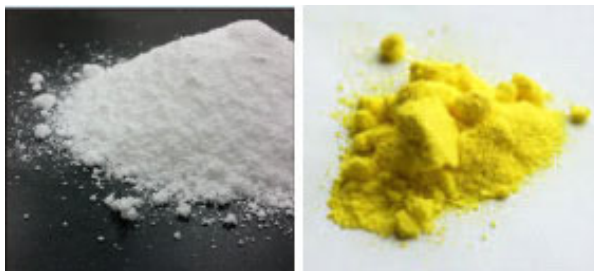
Fig. 2 Polymer Modified Warm Mix Asphalt Additive (PWMA) and Indonesian Natural Sulfur
