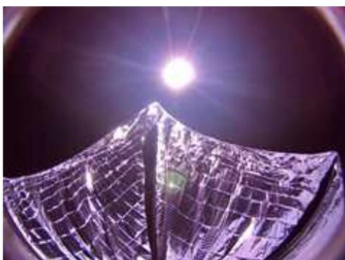
Fig. 8. Solar Sail Deployment Test of LightSail-1[15]
