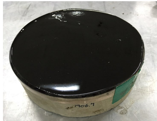
Fig. 8. Specimen for Resist Chloride Ion Penetration Test
