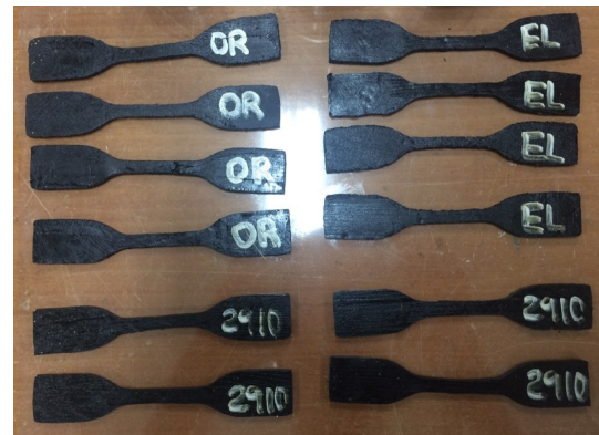
Fig. 2. Specimen for Elongation Test
