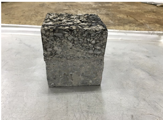
Fig. 4. Specimen for Shear Bonding Test
