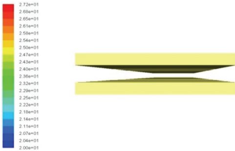
Fig. 13. Temperature distribution of magnet for air natural convection analysis.
