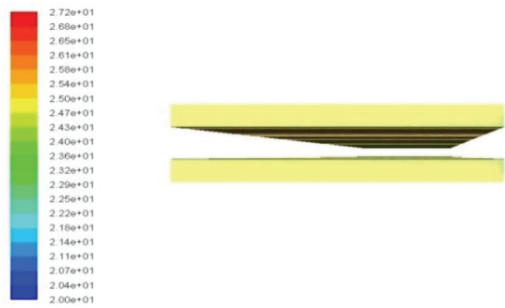
Fig. 11. Temperature distribution of magnet for air thermal conductivity analysis.
