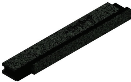
Fig. 9. Mesh for air thermal conductivity analysis.
