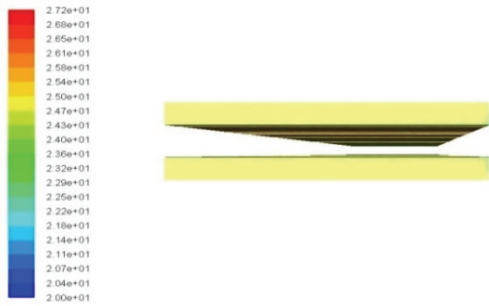
Fig. 15. Temperature distribution of magnet for 0 L/min flow rate.
