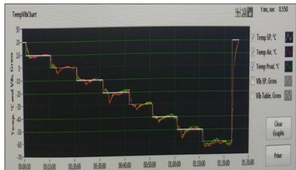
Fig. 7. Cold Step Test Result(Temperature)
