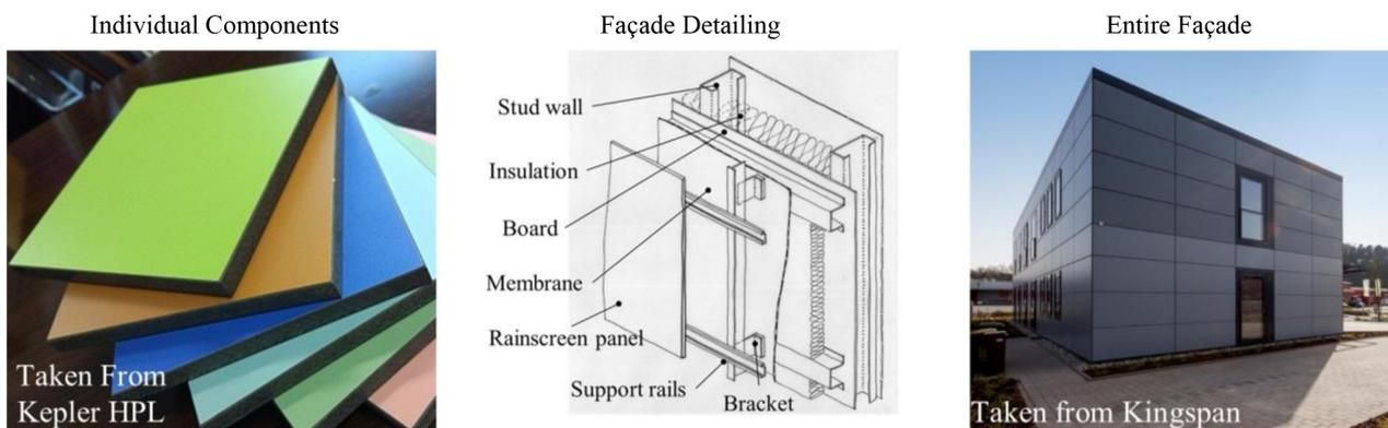
**Figure 2.** Images demonstrating the different levels of analysis when considering a façade. Currently, fire research focuses mainly on individual components, while large scale fire testing is used to assess façade systems.
