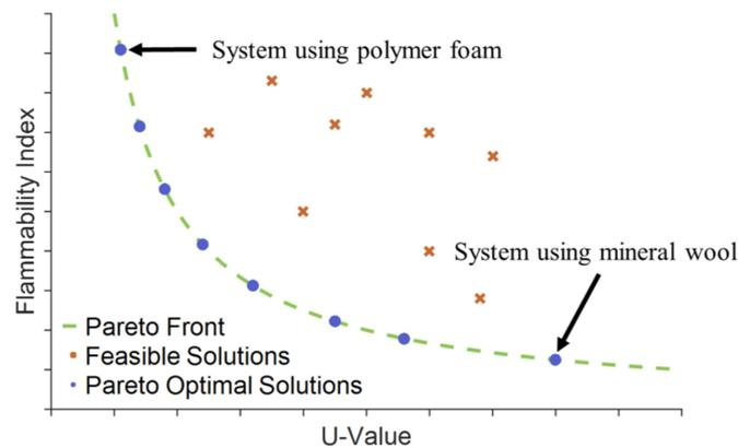
**Figure 7.** Example of a Pareto front, minimizing flammability vs. U-Value. Each solution represents a particular façade system design. Crosses represent solutions that are feasible, but not optimal. Labels show where hypothetical systems using polymer foam or mineral wool insulation might fall. The “flammability index” plotted in (c) is a hypothetical variable that quantifies the flammability of a façade. Currently, no such variable exists, but our research aims to create one.
