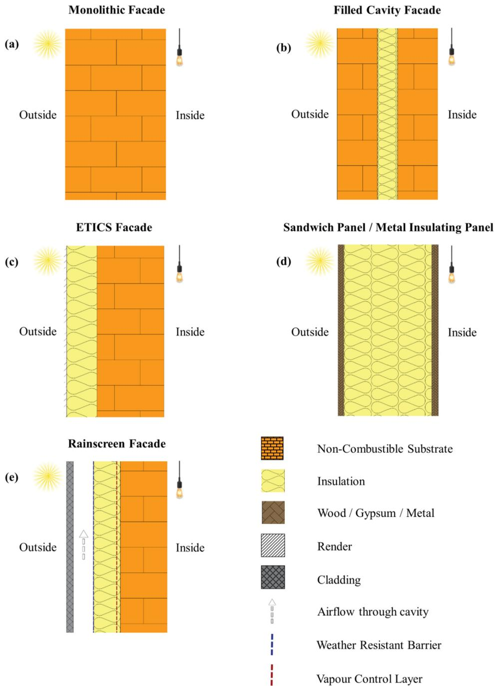
**Figure 5.** Simplified sections of common façade systems: (a) Monolithic Façade, (b) Filled Cavity Façade, (c) External Thermal Insulating Composite System (ETICS) Façade, (d) Sandwich Panel (or Metal Insulated Panel), (e) Rainscreen Façade. Note: The vapor control layer and weather resistant barrier in (e) are shown on the warm side of the insulation, for a climate that has an annual desire for vapor to flow from inside to outside.
