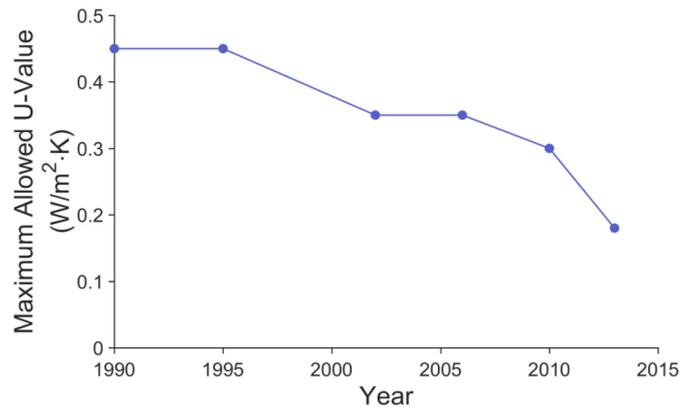
**Figure 3.** Maximum U-Values allowed for external walls in progressive editions of the UK building code. The U-Value of a wall quantifies its overall thermal resistance - a lower value indicates a better insulating performance (HM Government, 2016).
