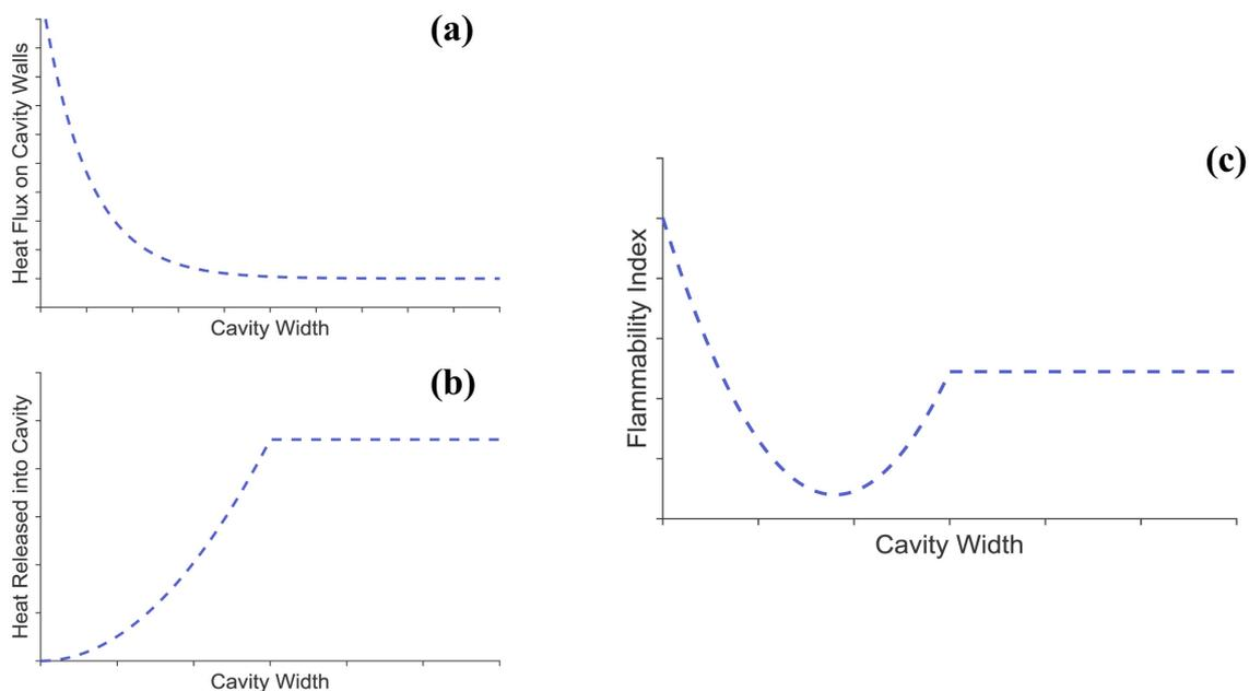
**Figure 6.** Plots illustrating how cavity width could hypothetically affect: (a) the heat flux on the cavity walls (radiation enhancement), (b) the heat released into the cavity (chimney effect), and (c) the total flammability (combination). The “flammability index” plotted in (c) is a hypothetical variable that quantifies the flammability of a façade. Currently, no such variable exists, but our research aims to create one.
