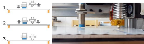
Fig. 2 Semi-automatic leveling method
