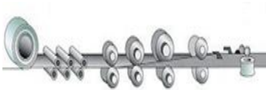
Fig. 2 A diagram of the real time smart roll forming stage and the section design
