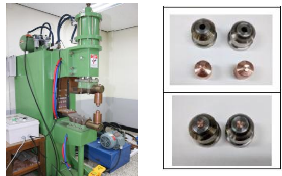
(a)AC Spot welding machine (b) heating dies and copper electrodes
